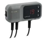
It is designed to control the water pump in the central heating and hot water circulation. It also works as a safety thermostat. It has the ability to turn on and off the pump. The pump will start after exceeding the temperature set by the user "C", and will turn off after exceeding the set off temperature "U".
