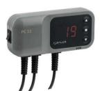
It is designed to control the water pump in the central heating circuit. The task of the device is to turn on the pump if the temperature exceeds the desired value and turn it on if the boiler cools down (due to shutting down). This prevents unnecessary pump operation and extends its life, which saves electricity.
