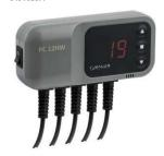
The controller turns on when the boiler temperature exceeds the user-set central heating pump activation temperature. The DHW pump works on the basis of a temperature difference. The DHW pump is switched on when the boiler temperature exceeds the tank temperature by the hysteresis set by the user. The hot water pump works until the boiler and tank temperatures equalize or the set tank temperature is reached.
